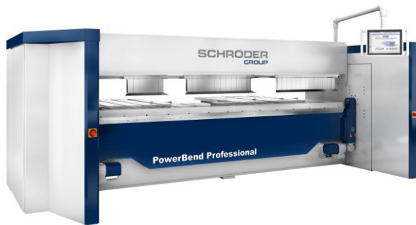
Figure 9: Example of a folding machine with emergency stop button on both machine columns (left, right)
