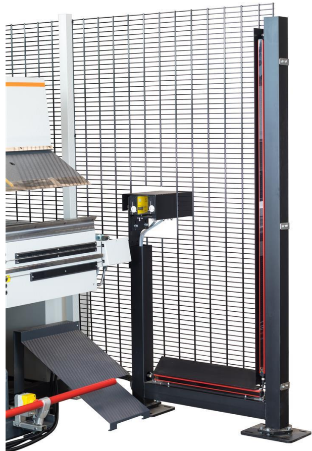
Figure 14: Example long folding machine as double bend with vertical and horizontal light curtain as access protection and step-behind protection as well as protective fence and laser beams (compare chapter 3.1.4)
