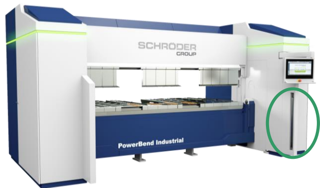
Figure 12: Example folding machine, front side, safeguarded by a light curtain (green circle)
