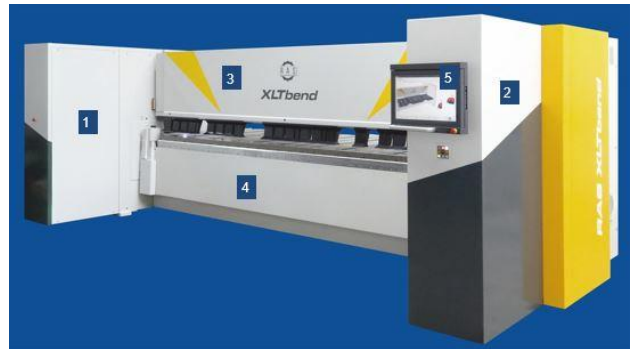
Figure 4: Example of a folding machine with segmented bending bar (front) on the upper beam
