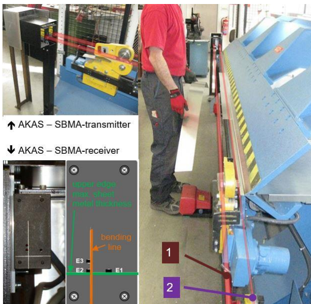
Figure 11: Example of laser protection with AKAS-SBMA during cutting process. Light beam 1 is active during cutting process and light beam 2 for inserting and clamping the sheets [12]
