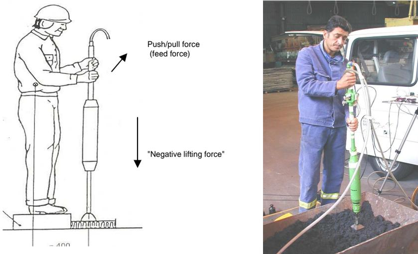
Figure 10 - Constraints upon recording of the feed forces
