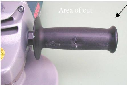
Figure 8 - Auxiliary handle of the angle grinder
