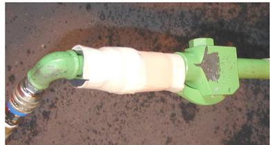
Figure 7 - Modified handle of the stamp hammer
