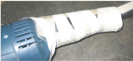
Figure 6 - Modified handle of the angle grinder
