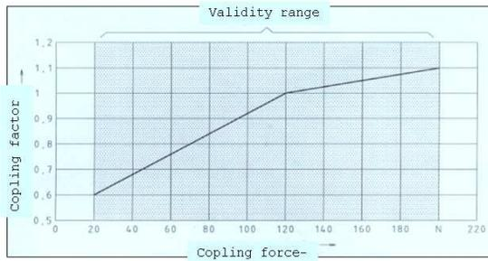
Figure 1 - Influence of the coupling forces to DIN 45679
