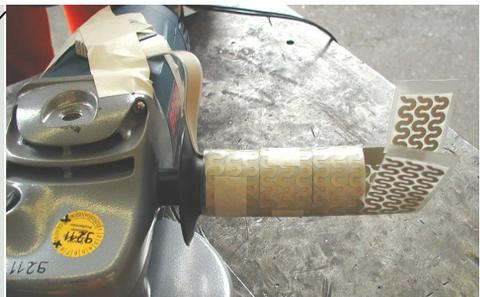
Figure 9 - Fitting the “finger matrix” to the auxiliary handle of the angle grinder
