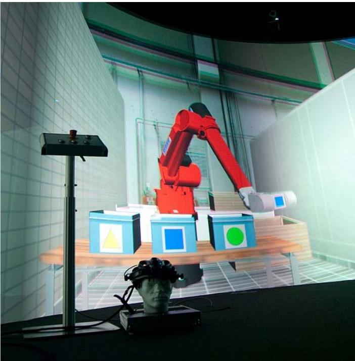
Figure 2: Projection wall, control panel and systems for recording of body and eye movement, in a scenario for human-robot interaction at the virtual workplace
