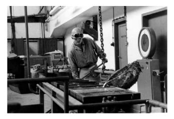
Metal pellets containing cadmium in ingot casting
