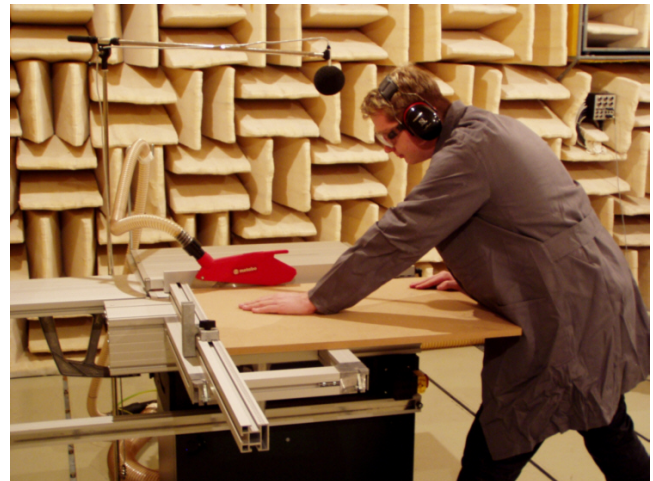
Measurement of noise emissions during sawing in the semi-soundproof chamber
