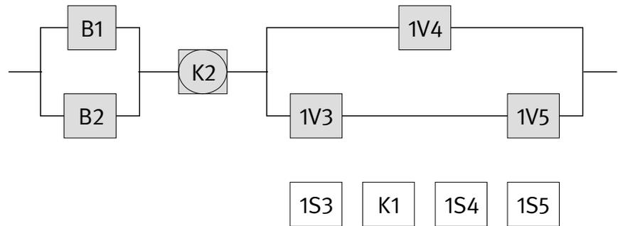
the same time, pressure builds up at the end of the cylinder above the piston, whilst the end below it remains shut off by 1V5. Owing to the pressure ratio in the cylinder, the pressure-relief valve 1V6 then opens and the ram of the press drops.
