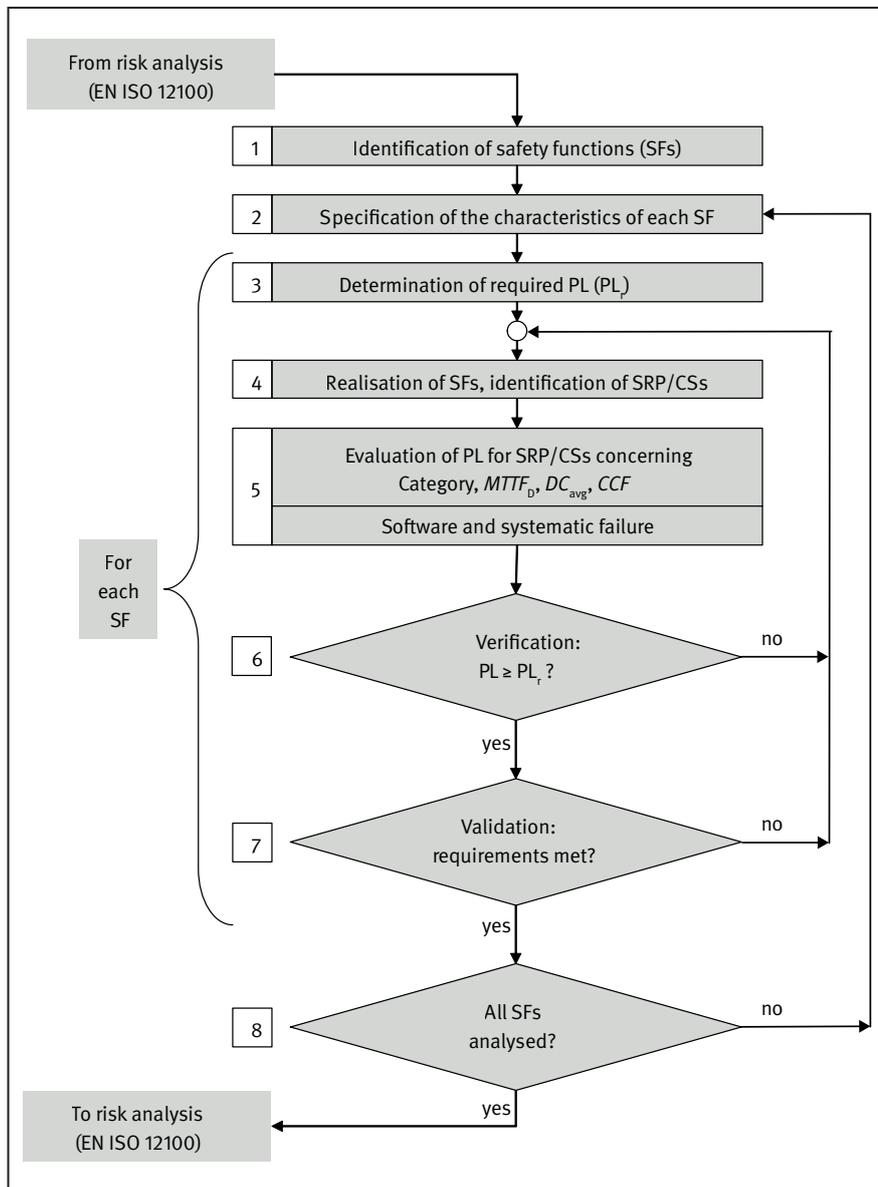
Figure 4.1: Iterative process for the design of safety-related parts of control systems: SF = safety function; PL = Performance Level;  $PL_r$  = required Performance Level; SRP/CS = safety-related part of a control system;  $MTTF_D$  = mean time to dangerous failure;  $DC_{avg}$  = average diagnostic coverage; CCF = common cause failure
