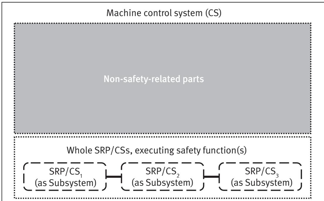
Figure 6.2: SRP/CS and sub-systems within the machine control system
