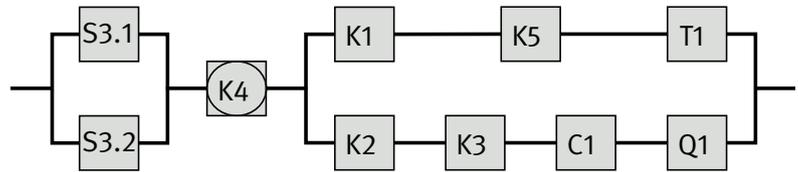
initiates a braking timer; upon timeout of the braking timer, the actuating signal for the mains contactor Q1 is interrupted. The timer setting is selected such that under unfavourable operating conditions, the machine movement is halted before the mains contactor Q1 has dropped out.
