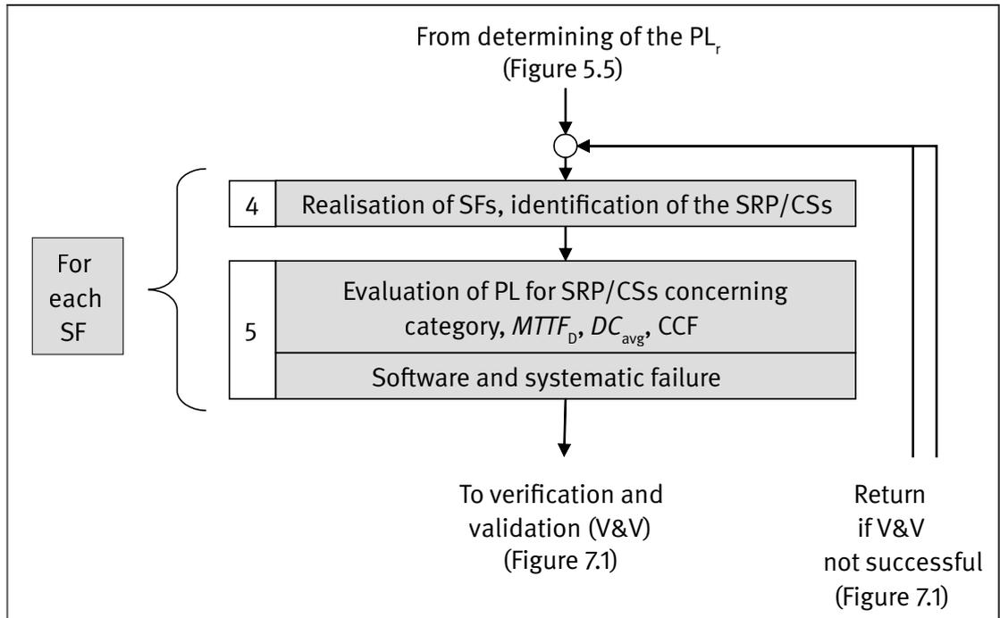
Figure 6.1: Determining of the attained PL in the implementation phase of the SRP/CS: excerpt from the iterative design process, see Figure 4.1
