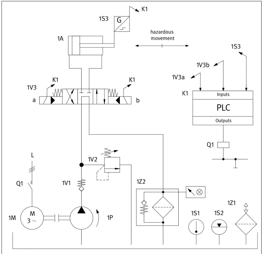
Figure 8.23: Hydraulic valve with electronic testing for the control of hazardous movements
