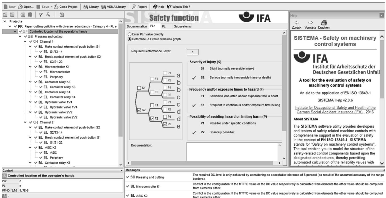
The area below the tree view shows the main context information for the selected basic element. This information comprises the PL,  $PFH_D$ ,  $MTTF_D$ ,  $DC_{avg}$  and number of CCF points of the higher-level subsystem, and the PL, PL and  $PFH_D$  of the higher-level safety function (this applies, of course, only to basic elements on lower hierarchy levels). The consequences of changes in the displayed parameters are thus displayed immediately.
